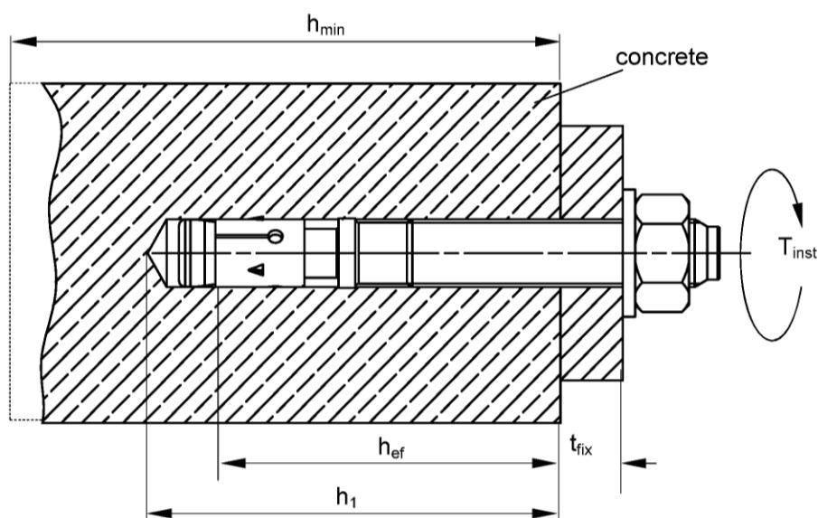
$h_{\text{ef}}$  = Effective anchorage depth
