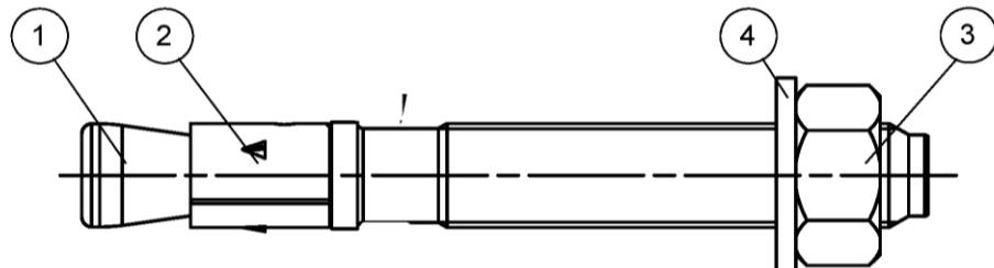
Cone bolt manufactured by turning:
