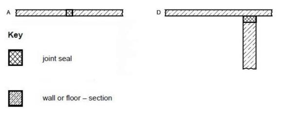
A tested linear joint in a horizontal test construction.
