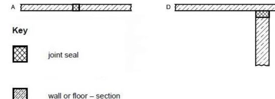
A tested linear joint in a horizontal test construction.
