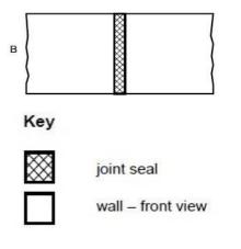
B tested vertical linear joint in a vertical test construction, and
