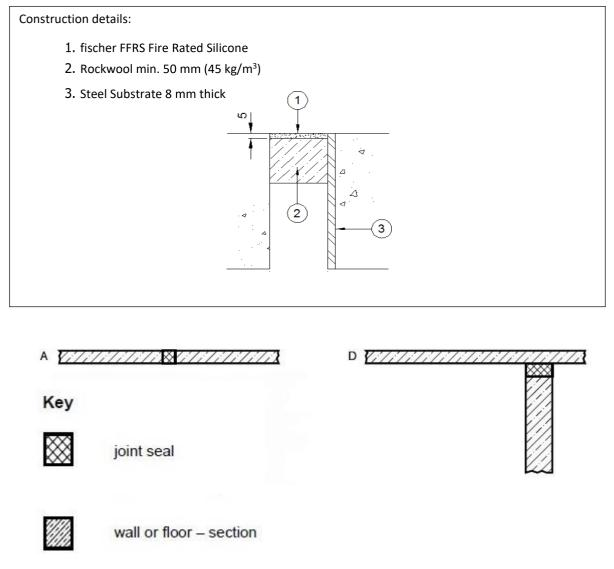
A tested linear joint in a horizontal test construction.
