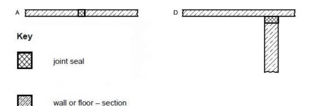
A tested linear joint in a horizontal test construction.
